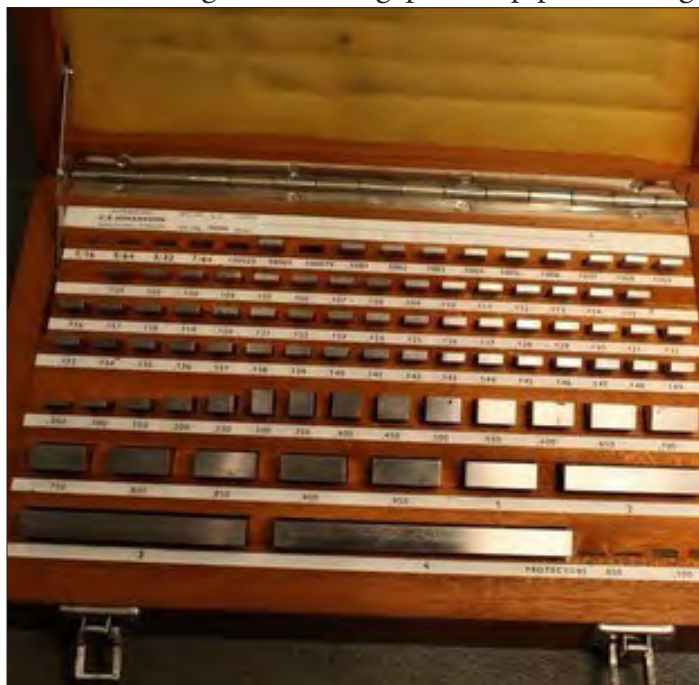
A set of precise pieces of perfectly flat, hardened steel known to this day as gauge blocks, or Jo blocks
